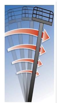
One of the biggest risks in using boom-type platforms is being catapulted out of the basket. This can happen easily if the boom swings, jolts or tilts away from the machine's centre of gravity..
